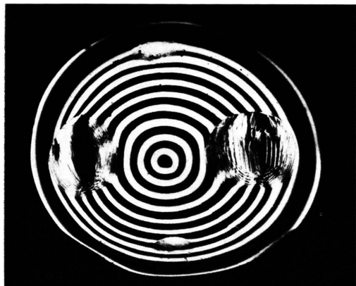
Fig. 1. Micrograph of a spherical gold crystal with (111) areas (larger systems) and (001) areas (smaller) systems [9].
